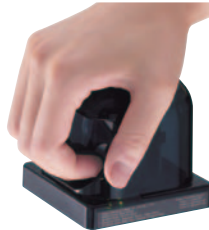
Detection only operates when fingers are bent in and lightly grip onto the unit.
