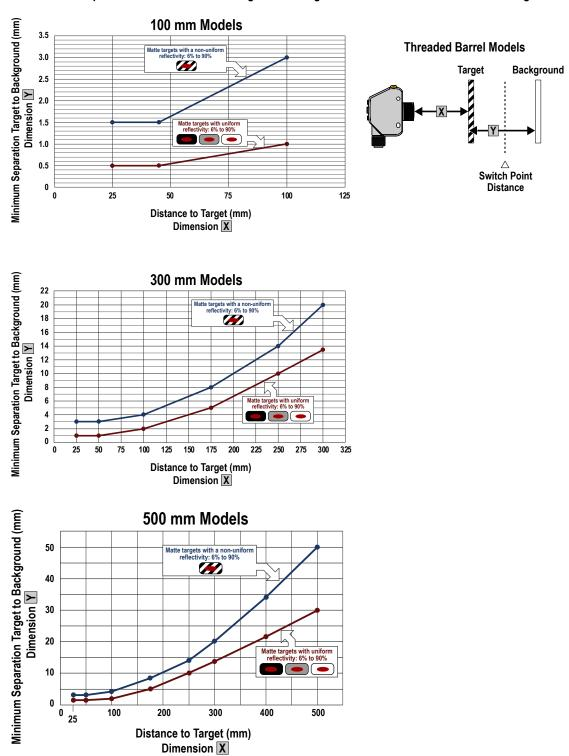
Minimum Separation Distance Between Target and Background for: Uniform and Non-Uniform Targets
