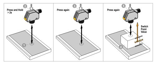
Figure 15. Two-Point Static Background Suppression (Light Operate shown)
