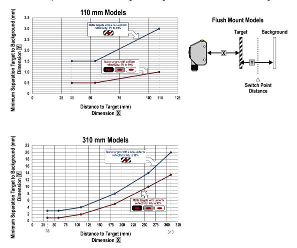
Minimum Separation Distance Between Target and Background for: Uniform and Non-Uniform Targets
