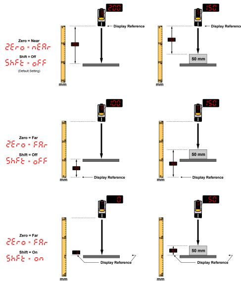
Figure 13. Example Zero and Shift settings
