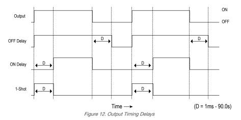
When one of the timing delay options is chosen, the sensor returns to the Setup menu and additional options become available to set the parameter(s):
