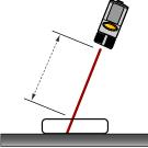
SOLUTION: Move the target closer to the sensor
