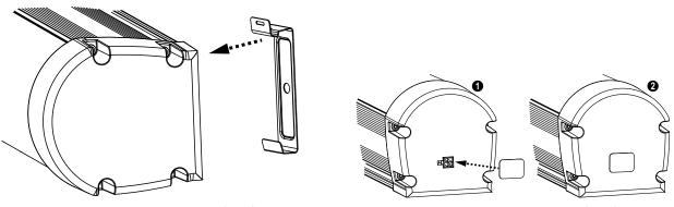
Figure 1. Attaching the snap brackets (step 6)
