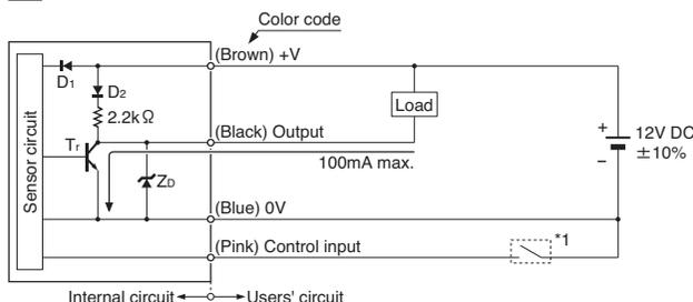
Symbols ... D<sub>1</sub>: Reverse supply polarity protection diode
