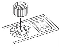
Aligning the marks accurately, press in the knob with force.
