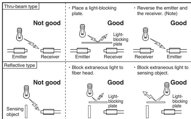
Note: Take care that extraneous light does not enter the receiver after being reflected from the sensing object.
