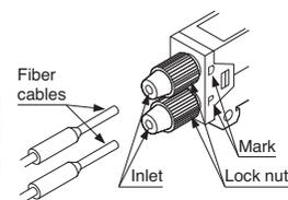
Note: Such as, **FD-G500**, insert the single-core fiber cable into the beam-emitting inlet and the multi-core fiber cable into the beam-receiving inlet. If they are inserted in reverse, the sensing accuracy will deteriorate.
