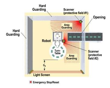
Figure 27. Supplemental safeguarding inside a robotic work cell
