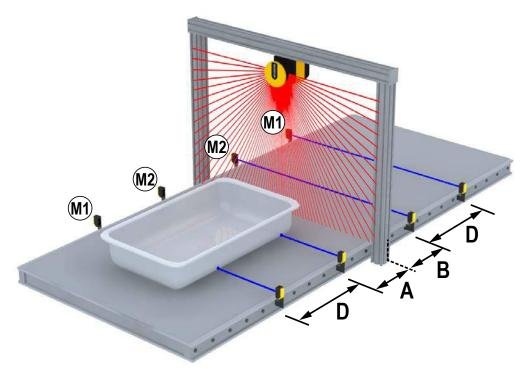
Figure 43. Muting function in the T configuration
