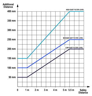
Figure 21. Additional distance for 70 mm resolution
