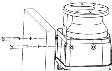
Figure 31. Mounting the scanner directly to a surface
