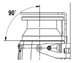
Figure 34. Adjust the scanner angle
