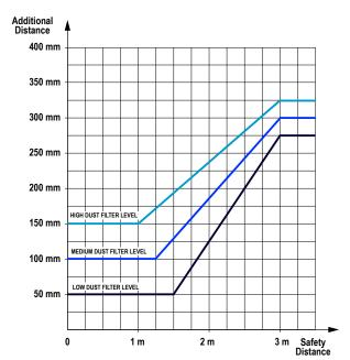
Figure 22. Additional distance for 40 mm resolution
