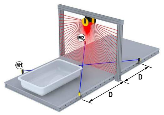
Figure 42. Muting function in the X configuration
