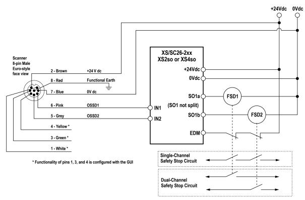
Figure 39. Wiring to a Safety Controller
