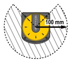
Figure 24. Limited detection capability zone
