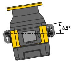
Figure 35. Adjust the roll angle
