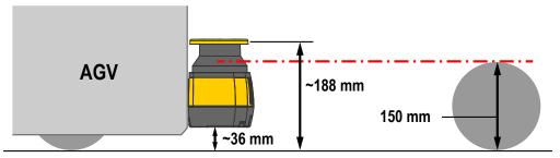
Figure 30. Diagram to determine the additional distance with lack of floor clearance
