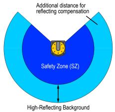
Figure 23. Reduce or remove a highly reflecting background
