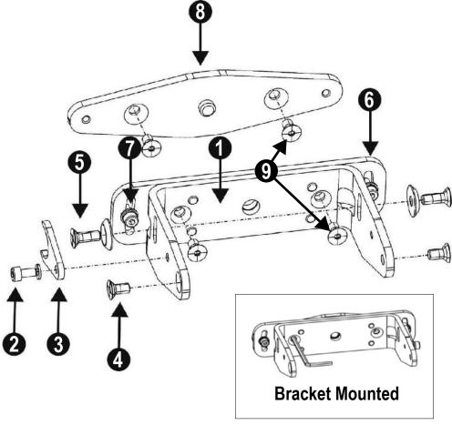
Figure 33. Pitch and roll angle adjustment bracket (SXA-MBK-1)
