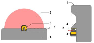
Figure 14. Mounting the scanner recessed into the machine
