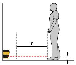
Figure 26. Calculating the safety distance for each resolution
