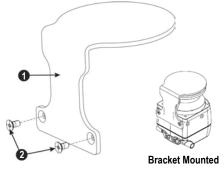
Figure 32. Mounting the protection bracket to the scanner
