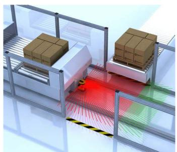
Figure 7. Mobile area guarding on AGVs
