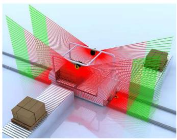
Figure 9. Mobile area guarding with side vertical guarding
