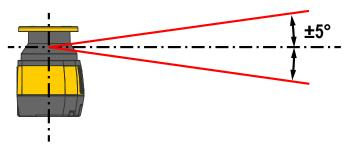
Figure 20. Position the scanner to avoid light interference
