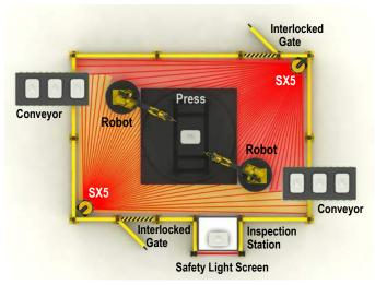
Figure 6. Stationary area guarding with multiple scanners
