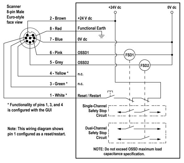
Figure 37. Wiring with FSD inputs
