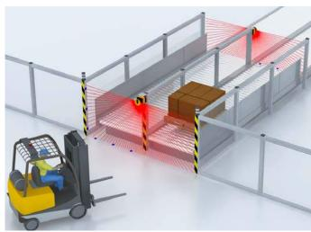
Figure 8. Vertical guarding with reference contour monitoring
