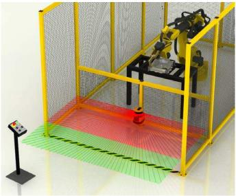
Figure 4. Horizontal stationary area guarding
