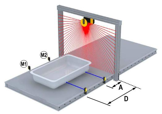
Figure 44. Muting function in the L configuration
