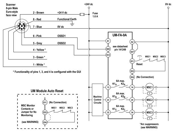
Figure 38. Wiring using a UM module
