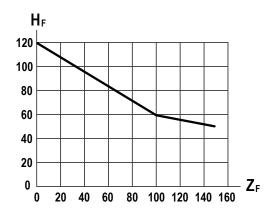
Figure 29. Diagram to determine the additional distance  $Z_F$  with lack of floor clearance  $H_F$
