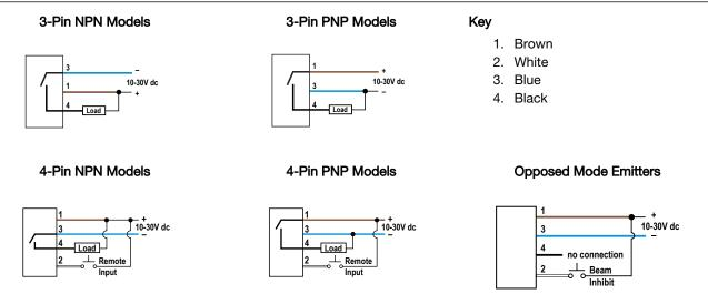
Note: All 4-pin and cabled models have a remote input on the white wire (pin-2).
