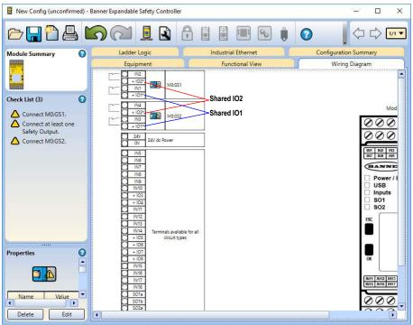
Figure 4. Wiring Diagram Tab View of Shared I/Os
