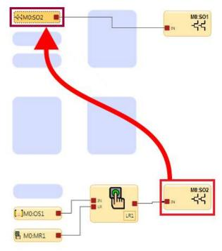
Figure 107. Safety Output controlled by another Safety Output
