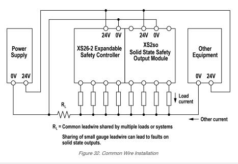
**Note:** When the Safety Output turns Off, the voltage at that output terminal must drop below 1.7 V with respect to the 0 V terminal on that module. If the voltage is higher than 1.7 V, the Safety Controller will decide that the output is still on, resulting in a lockout. Consider using larger gauge wires, shorter wires, or using a single point grounding scheme similar to what is shown in the following diagrams.
