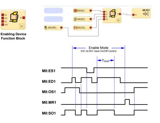
Figure 61. Timing Diagram – Enabling Device, Simple Configuration
