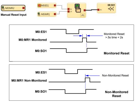
The Manual Reset input device can be configured for one of two types of reset signals: Monitored & Non-Monitored
