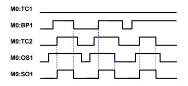
The Two-Hand Control actuators TC2 and the Bypass Switch BP1 need to be in the Run state and need to be the last devices in time to transition to the Run state for the TC1 function block to turn On.
