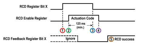
Figure 23. Virtual Reset or Cancel Delay (RCD) Sequence – Timed Method
