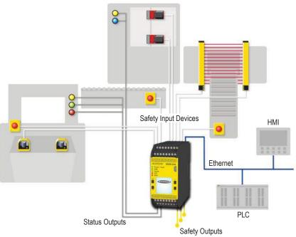
Figure 2. Safety Outputs (Example Application)
