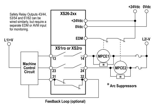
Figure 40. Generic XS/SC26-2 Hookup: Safety Relay Output (Dual-Channel) with EDM
