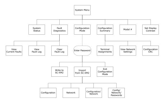
Figure 108. Onboard Interface Map
