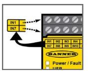
Figure 13. XS/SC26-2 Input and output terminal locations
