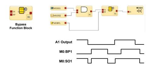
Figure 58. Timing Diagram-Bypass Block
