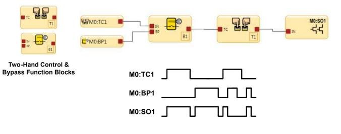
If both TC1 actuators and the BP1 Bypass switch active at the same time, the B1 Bypass function block output and the Two-Hand Control function block output turn Off. The outputs for B1 and T1 will only turn On when either the TC1 actuators or the BP1 switch are in the Run state.
