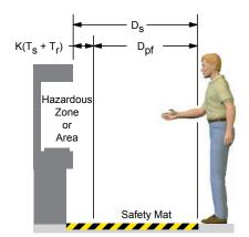
Figure 16. Determining safety distance for the safety mat
