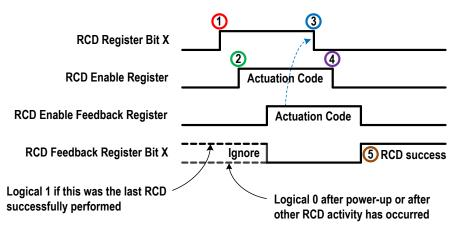
Figure 22. Virtual Reset or Cancel Delay (RCD) Sequence – Feedback Method
