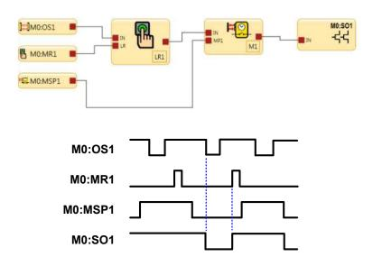
When a safeguarding device OS1 transitions to a Stop state in a valid muting cycle, the latch reset function block will latch and require a reset signal to keep SO1 on after muting ends.
