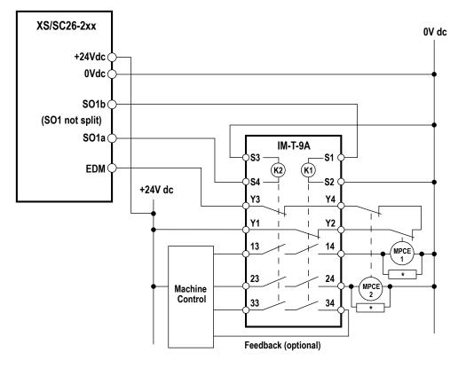
\* Installation of transient (arc) suppressors across the coils of MPCE1 and MPCE2 is recommended (see Warning)
