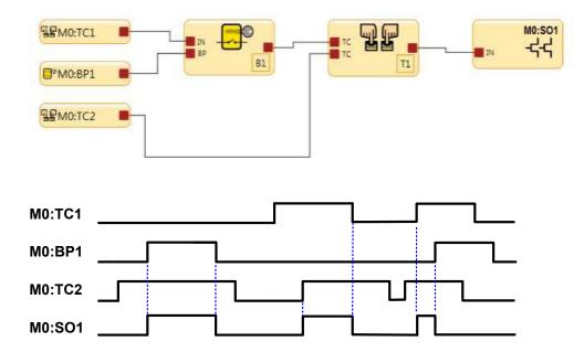
The Bypass function can be used with the TC2 actuators to turn the Safety Output On.
