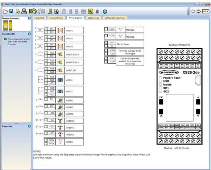
Figure 84. Wiring Diagram Tab-XS26-2
