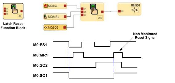
The Latch Reset function block LR1 will turn its output and the safety output SO1 Off when the E-Stop button changes to the Stop state.
