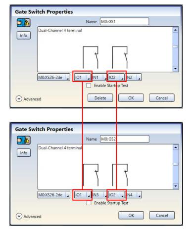
Figure 3. GS1 and GS2 Sharing IO1 and IO2
