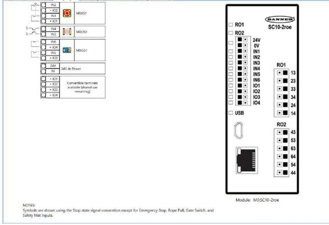
Figure 109. Wiring Diagram tab with an E-stop button, optical sensor, and gate switch
