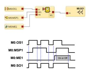
Figure 74. Timing Diagram-Two-Way Muting Block, One Muting Sensor Pair
