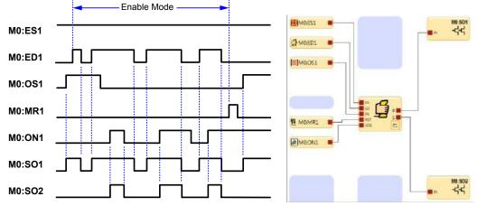
E1 enabling mode starts when the Enabling Device ED1 is switched to the Run state. ED1 and ES input devices have On/Off control authority while in Enable mode. When MR1 is used to perform a reset, the normal Run mode is re-established and OS1 and ES1 have the On/Off control authority.
