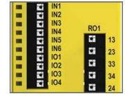
Figure 14. SC10-2 Input and output terminal locations
