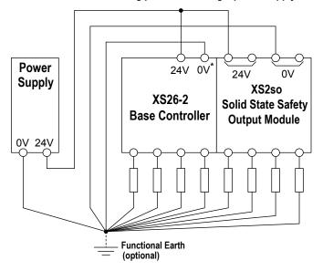
Preferred 0V routing plan when a single power supply is used
