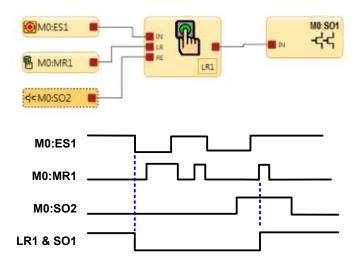
When output SO2 is On, the SO2 reference signal state is On or High. The function block above shows reference signal SO2 connected to the Reset Enable node RE of Latch Reset Block LR1.
