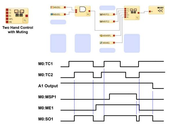
Actuators TC1 and TC2 can initiate a two-hand cycle if the mute enable ME1 is not active. ME1 must be active for the MSP1 mute sensors to keep the SO On after the TC1 and TC2 actuators are in the Stop state.
