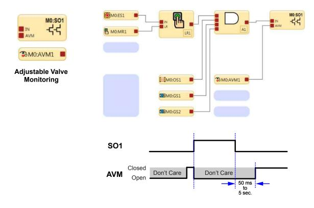
Adjustable Valve Monitoring AVM is a way to check the operation of dual channel valves. The force guided N.C. monitoring contacts of the valves are used as an input to detect a "stuck on" fault condition and will prevent the safety controller outputs from turning On.
