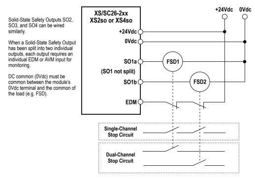
Figure 39. Generic XS/SC26-2 Hookup: Solid-State Safety Output with EDM
