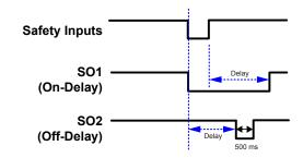
Figure 28. Timing Diagram – General Safety Output On-Delay and Off-Delay
