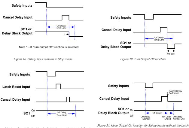
Figure 20. Keep Output On function for Safety Inputs with the Latch Reset
