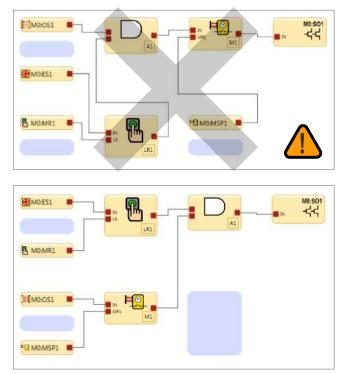
Figure 76. Emergency Stop and Mute Function
