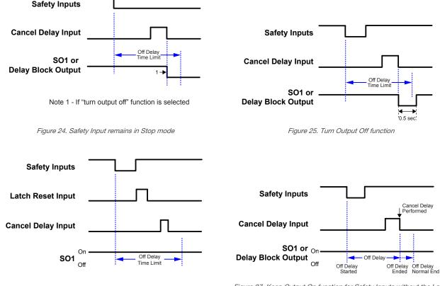
Figure 26. Keep Output On function for Safety Inputs with the Latch Reset
