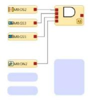
Figure 66. Latch Reset and Referenced Safety Output and AND block
