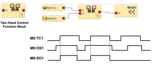
Either the TC1 input or the OS1 input has turn Off authority. OS1 needs to be in the Run state before TC1 can turn the output of T1 & SO1 On.
