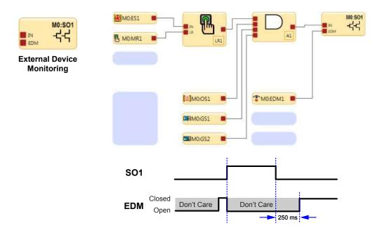
External Device Monitoring EDM is a way to check the operation of dual channel final switching devices or machine primary control elements. The force guided N.C. monitoring contacts of the FSD or MPCE are used as an input to detect a "stuck on" fault condition and will prevent the safety controller outputs from turning On.
