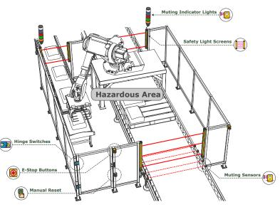
Figure 11. Sample Application - Robotic Cell
