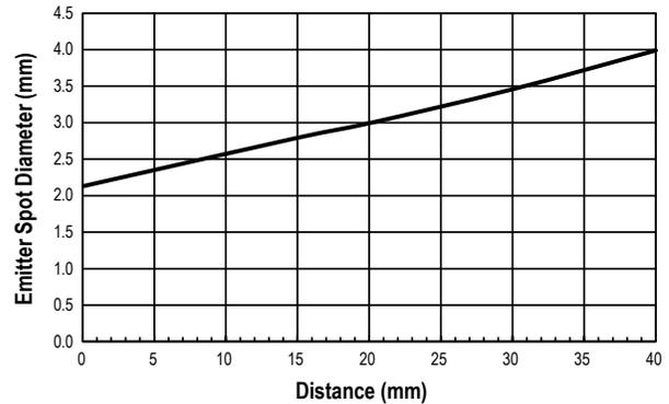
Figure 6. Typical Emitter Spot Diameter vs. Distance
