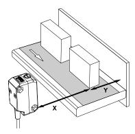
Figure 4. Background Suppression Mode Application Example
