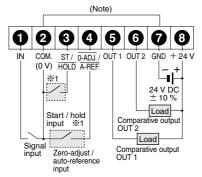
Note: COM. (0 V) is internally connected to GND.
