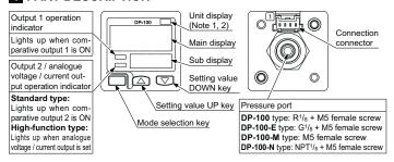
Notes: 1) In the case of a model that is intended for use outside Japan, attach the unit switch plate corresponds to the set pressure unit.
