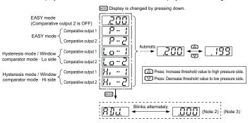
Notes: 1) If the set pressure range is exceeded, " !!/" " (exceeds the upper limit) or " #@##" (exceeds the lower limit) will appear on the sub display. " #@##" will also appear if the Hi side threshold value exceeds the Lo side threshold value when setting the "hysteresis mode / window comparator mode" threshold value.
