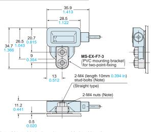
Note: M4 stud-bolts have been welded to this unit. M4 nuts are not supplied with the sensor. Purchase it separately.
