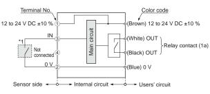
Note: The output does not incorporate a short-circuit protection circuit.
