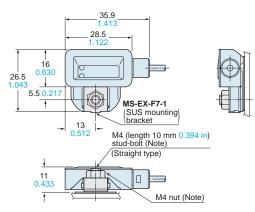
Note: A M4 stud-bolt has been welded to this unit. M4 nut is not supplied with the sensor. Purchase it separately
