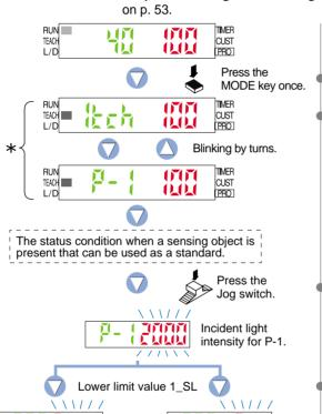
threshold value limits have been correctly set and the setting for 'lower limit value 1\_SL' (green) will be displayed.
