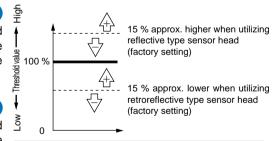
The threshold value is variable from approx. 5 % to 200 % (in increments of 1 %).
