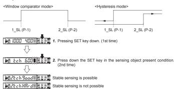
Note: If the value after setting exceeds the maximum (minimum), the maximum (minimum) sensitivity will be set
