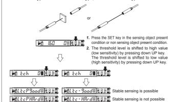
Note: The shift value of approx. 15% is an initial value. Display of the shift value can be changed to percentage (approx. 0 to 999% (unit 1 %)] or incident light intensity (0 to 9999 (unit 1))].
