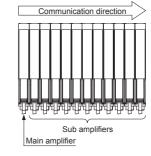
• When this product and other products (e.g. fiber sensor amplifiers, pressure sensor controllers, etc.) are connected together in cascade, install those products so that they are in order of Group A, B, D and C as shown in the right figure. This product is included in Group D.
