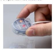
When conditions are normal Sensor light from the emitter is able to reach the receiver
