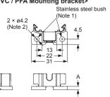
Notes: 1) Drawing above is for PFA mounting bracket. PVC mounting brackets M-SQ4-11, M-SQ4-21 and M-SQ4-23 do not incorporate stainless steel
