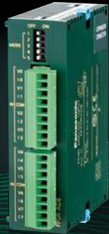
NEW Analog Input Unit Input: 8 channels AFP0RAD8
