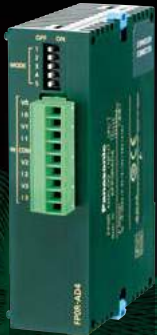
NEW Analog Input Unit Input: 4 channels AFP0RAD4
