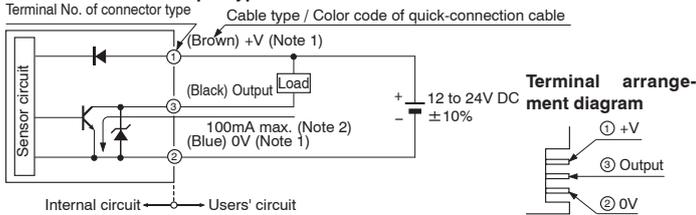
Notes: 1) The quick-connection sub cable does not have +V (brown) and 0V (blue). The power is supplied from the connector of the main cable.
