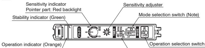
Note: The mode selected by the mode selection switch for FX-311B(P) and FX-311G(P) is 'LONG', 'STD' or 'FAST'.
