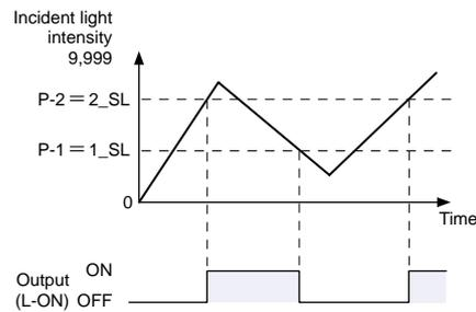
\* In this figure, the incident light intensity of P-1 is less than that of P-2.
