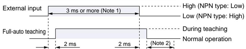
Notes: 1) Pass the sensing object past the sensor once while an input signal is being input.
