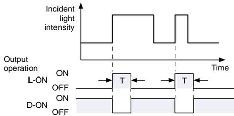
**When using trailing differential mode**
