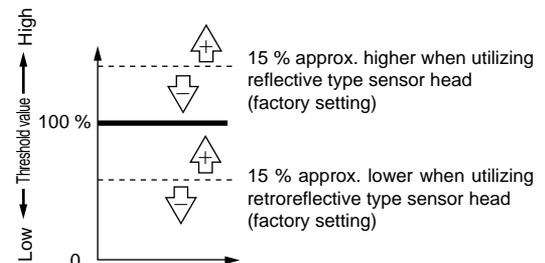
The threshold value is variable from approx. 5 % to 200 % (in increments of 1 %).
